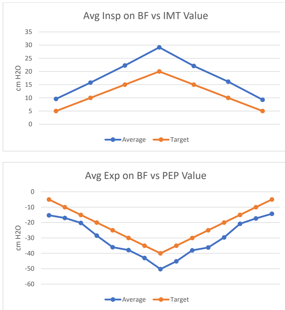
Figure 51 – Graphs of deviations of BreathForce prototype from IMT and PEP threshold valve values
