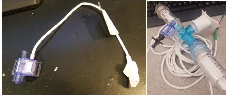
Figure 14 – (Top) PendoTech Pressure sensor. (Bottom) Pressure sensor and threshold devices attached to the breathing apparatus tee connector
